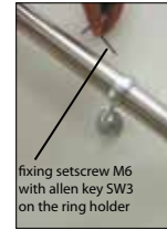
Clamp handrail at bracket
